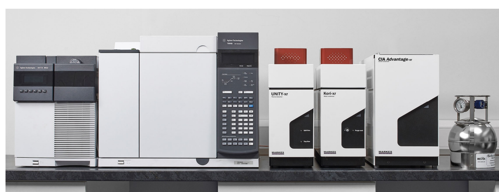
Figure 2: Markes and Agilent TD-GC-MS equipment configuration.
